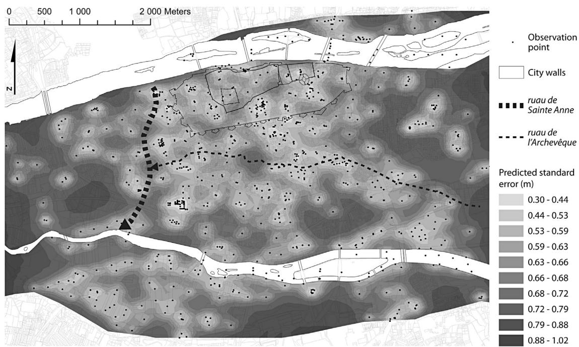
**Fig. 10.** Predicted standard error of the geostatistical model of the accumulated thickness of clayey-silty and clayey-peaty silt in the alluvial plain of Tours.
