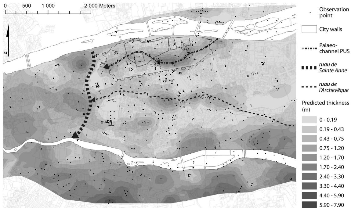
**Fig. 9.** Geostatistical model of the accumulated thickness of silty-clayey and peaty deposits in the alluvial plain of Tours ( $R^2$ : 0.61; mean standardized error: -0.002; average standard error: 0.91 m).
