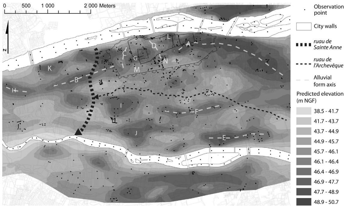
**Fig. 6.** Geostatistical model of the altitude of the top of the alluvium in the alluvial plain of Tours ( $R^2$ : 0.72; mean standardized error: 0.010; average standard error: 0.92 m). A: highest point of the top of the alluvium in the west part of the low fluvial terrace; B: natural levee; C, D: breach in levee; E, F: natural levee or point bar; G, H, I, J: natural levee or point bar intersected by thalwegs; K, L: Holocene island; M: protohistoric settlement; N: Roman baths.
