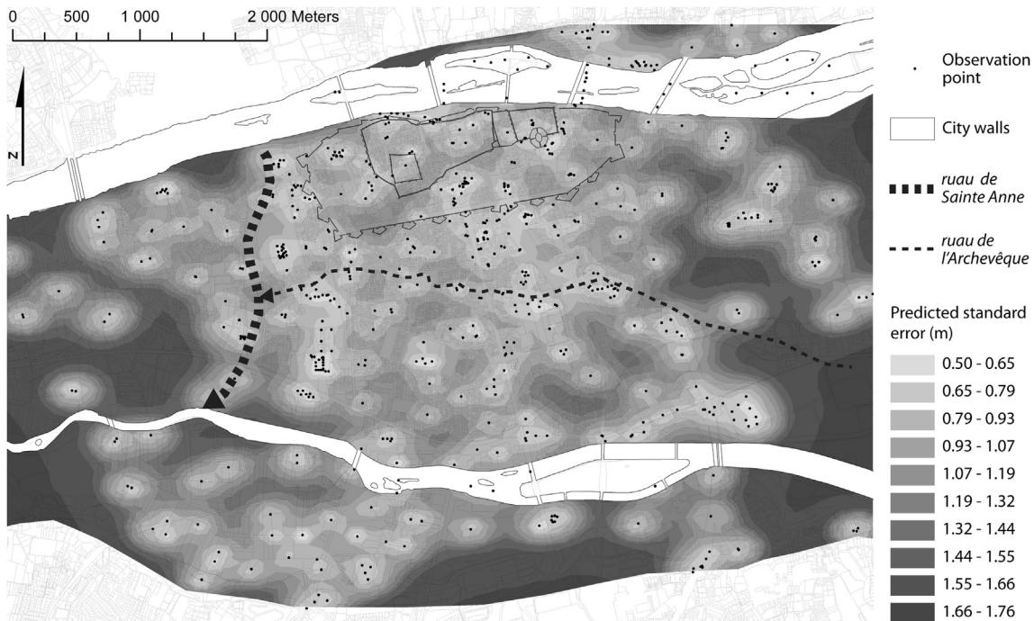
**Fig. 5.** Predicted standard error of the geostatistical model of the altitude of the top of the limestone bedrock of the alluvial plain of Tours.
