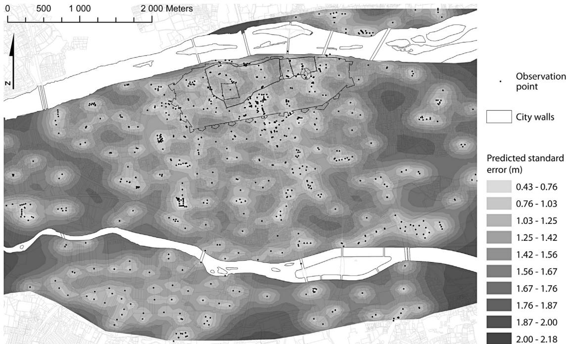
**Fig. 12.** Predicted standard error of the geostatistical model of the thickness of anthropogenic deposits in the alluvial plain of Tours.
