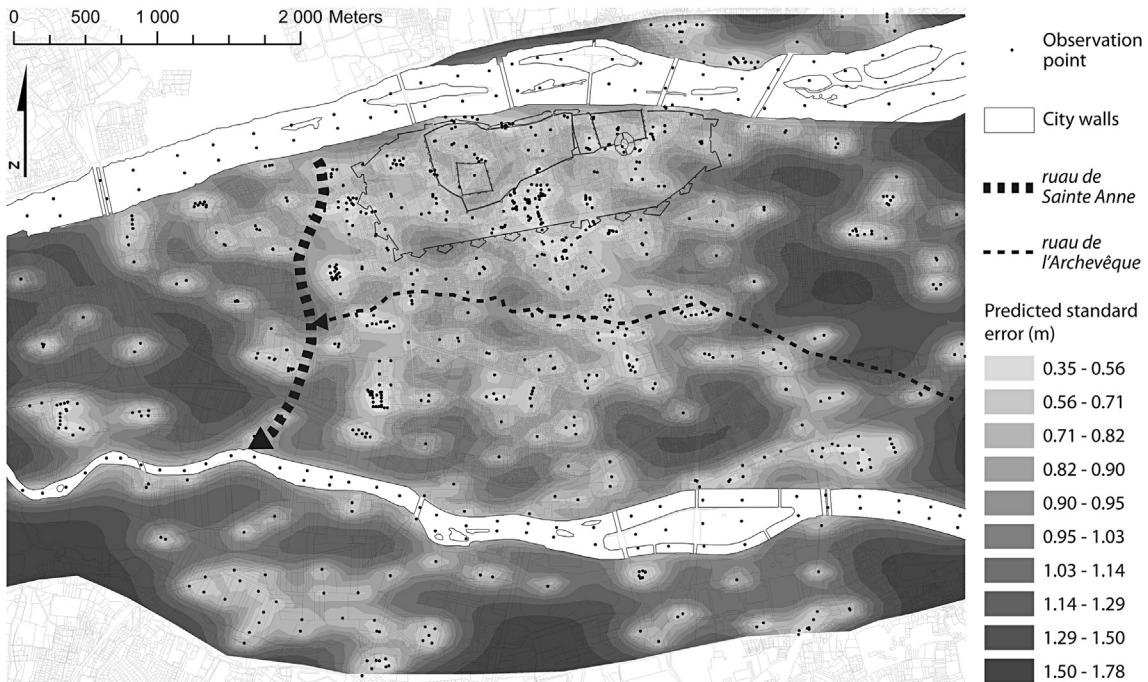
**Fig. 7.** Predicted standard error of the geostatistical model of the altitude of the top of the alluvium in the alluvial plain of Tours.
