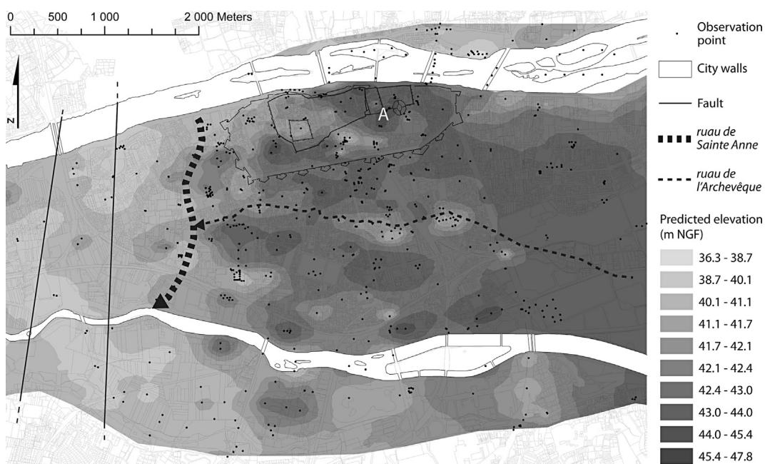
**Fig. 4.** Geostatistical model of the altitude of the top of the limestone bedrock of the alluvial plain of Tours ( $R^2$ : 0.58; mean standardized error:  $-0.001$ ; average standard error: 1.28 m). A: highest point of the top of the calcareous bedrock.
