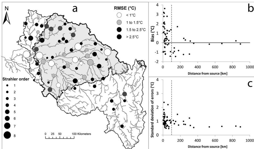
Figure 3. Thermal model performance at 67 measurement stations during the summer period between 2000 and 2006: (a) spatial distribution of root mean square error (RMSE), (b) biases ( $T_{sim} - T_{obs}$ ) and (c) standard deviation of errors as a function of the distance from headwater
