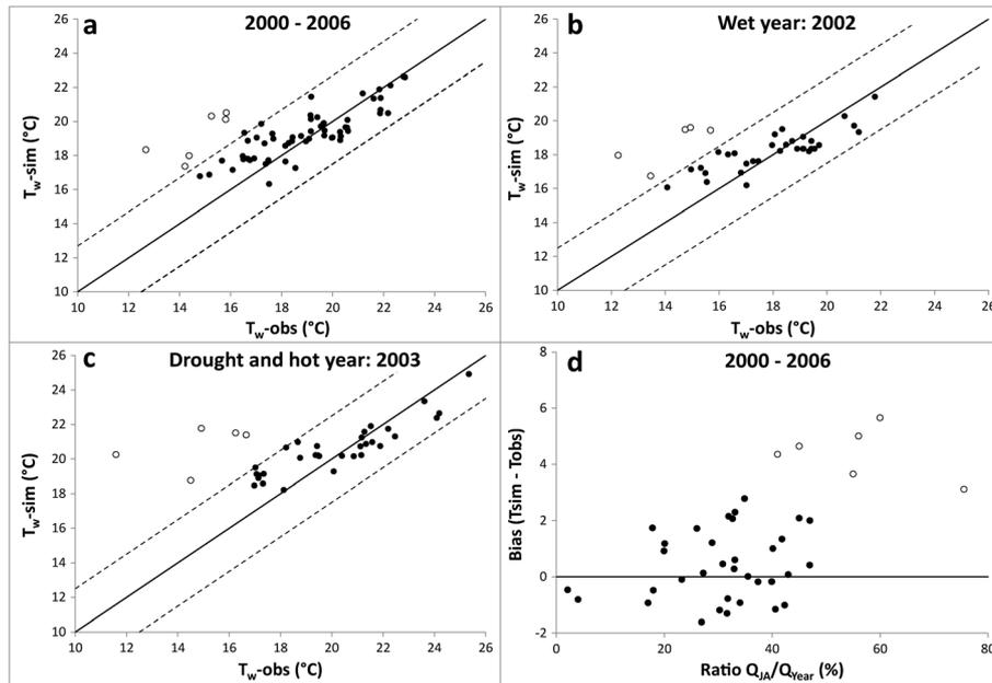
Figure 7. Simulated temperature as a function of observed temperature in summer 2000–2006 (a), in 2002 (b) and in 2003 (c). Dashed lines represent biases of  $\pm 2.5^\circ\text{C}$ ; (d) mean biases as a function of the ratio between the mean summer flow and the mean annual flow ( $Q_{JA}/Q_{Year}$ ) in summer between 2000 and 2006 (white circle: stations where  $T_w\text{-obs}$  is outside the uncertainty area; black circle: other stations)
