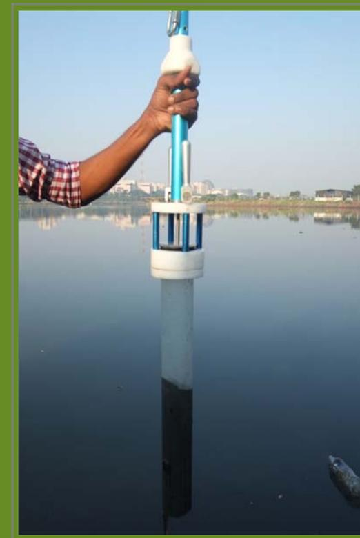
Bed sediments of the coum river retrieved with an uwitec coring device. The water quality is studied through the concentration of trace elements and organic compounds
